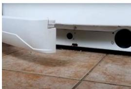
Some water will leak out when you remove your filter, so put some towels down to protect your floor. Unscrew the filter and let the water flow out.
