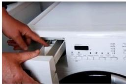
To do a proper clean, you'll need to completely pull out the drawer. It should be easy to do this. Simply pull the drawer out as far as it can go, then look for a catch to press down that lets you remove it from the machine. In most models it's right in the middle - if you can't see it, check out the manufacturer's instructions.
